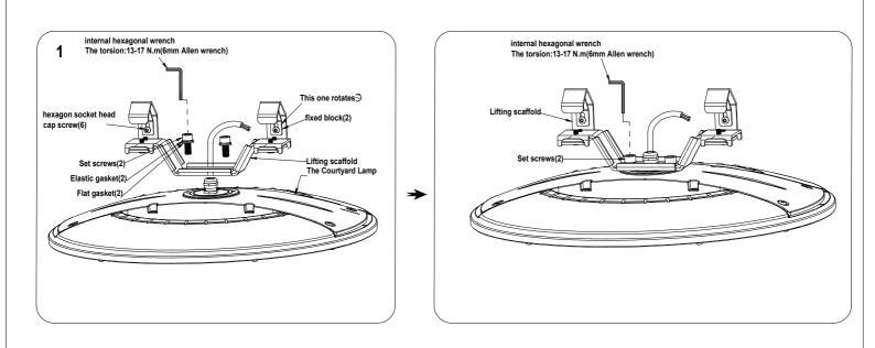
Step 2:The lifting bracket is fixed on the lamp body and then hung on the wire rope.
