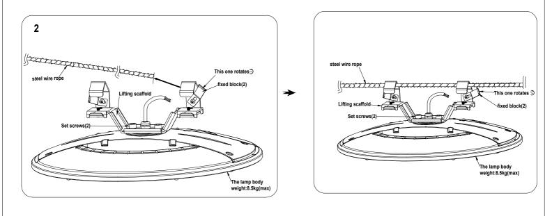
Step 3: pass the wire rope through the lifting bracket, adjust the position of the fixing block, and tighten the screws with the hex wrench to fix the position
