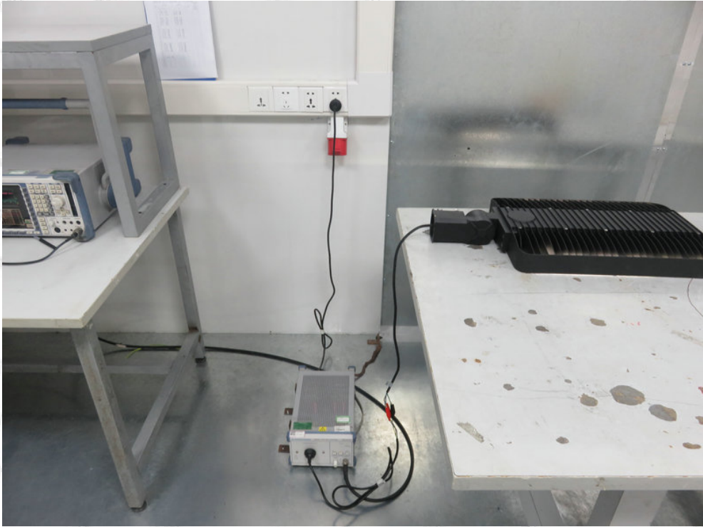
Photo of Power Line Conducted Emission Test
